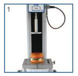
The texture analyzer's crosshead moves in either an up or down direction to compress or stretch a food sample. The moving crosshead is fitted with a load cell to measure the foods force response to the deformation.
