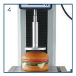
The crosshead then returns and the sample responds to the conditions created. Forces are manipulated through the use of probes and fixtures recreating conditions that the food is exposed to during mastication or handling.
