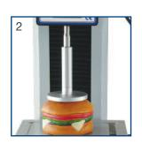
In a compression test, the load cell acts just like an upside down laboratory balance. Data collection can be "triggered" to begin when the sample's surface is detected giving a constant start point to repetitive tests.
